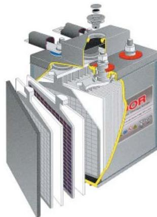
Plate thickness in this type of cell is determined by the application it is used in; long discharge durations require a thicker plate than high power rapid discharges which require thin plates.
